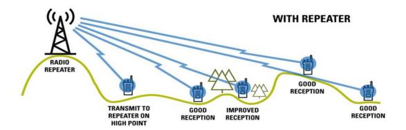
In the upper picture, not every radio gets good reception because of differences in the terrain. Trees absorb some of the signal and a hill blocks all reception. In the lower picture, the radio in the trees has an improved signal and the radio that had no signal before now has a good signal.
