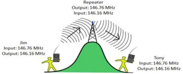
In the above example, Jim and Tony cannot talk directly to each other because the hill blocks the signals between their radios. The repeater at the top of the hill overcomes that limitation. Obstacles within the normal line of sight distance can also interfere with communication as shown below.
