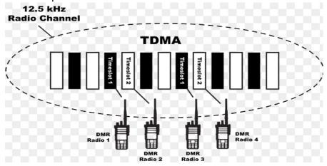
DMR transmissions have a 30ms window for each time slot. That window is further divided into a 27.5ms frame followed by a 2.5ms gap. For each 60ms, the radio is only transmitting for 27.5ms, which results in extended battery life and less heat.
