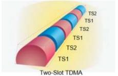
The channel bandwidth of DMR transmissions is half the size of standard analog FM transmissions (12.5kHz verses 25kHz) making it possible to accommodate more DMR channels in the same amount of spectrum space as standard analog FM channels.
